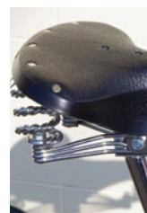
The saddle is Brooks' springiest. Getting it to stay at the right height required a new nut for the seat bolt, however
