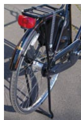
Massive (but malleable) steel carrier and stand. The chaincase is plastic, so not as rattly as you might imagine
