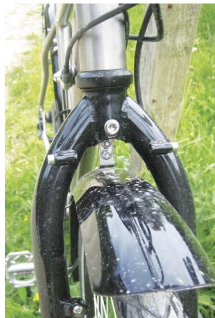
● (Above) Fork clearance is huge on the Ti Adventure, so the mudguard needs spacing down. A 54-57mm tyre will fit in underneath the mudguard. With the mudguard removed, it's possible to fit a 3in 29+ tyre – on a wider rim, of course
