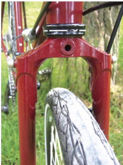
● (Above) The 26in-wheel Disc Trucker will take 2in tyres plus mudguards but comes with skinny 37mm tyres that actually measure 33mm. Bigger tyres would suit roughstuff and expedition tourers alike
