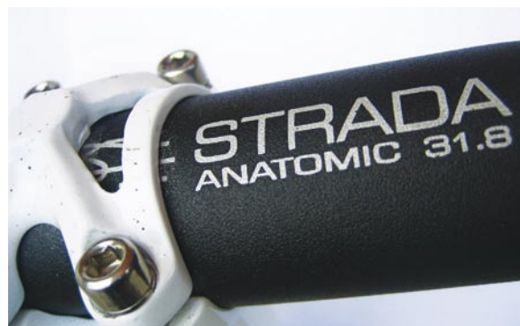
Modern bars and stems are mostly 31.8mm diameter at the stem clamp
