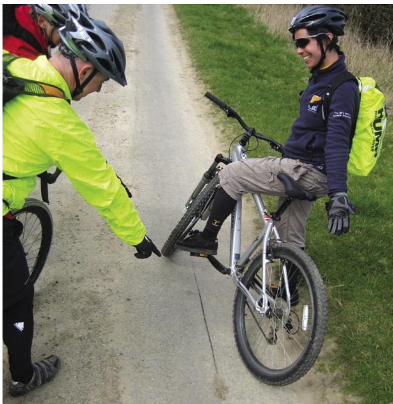
A back-wheel skid caused by too much rear brake and too little front. The front stops you quicker and without skidding – but not as quickly as car
