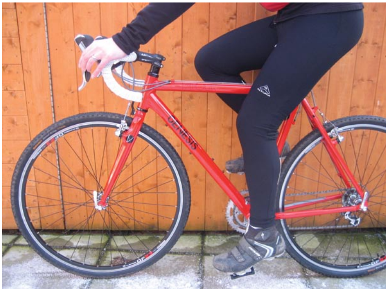
The no-nonsense way to set your saddle height. With the arch of your foot on the pedal, your leg is straight with cranks in line with the seat tube
